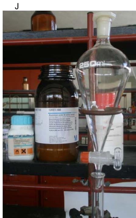
Elution of the column with 150mL of  $\text{CH}_2\text{Cl}_2$  (J)
