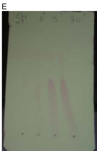
TLC visualization with UV lamp for circumferential marking of the benzoic acid spots with pencil (E)
