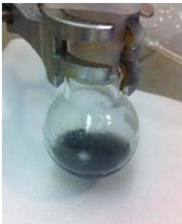
Figure SM 12.3.1.3 - Reaction mixture – decomposition of excess  $\text{H}_2\text{O}_2$  with  $\text{MnO}_2$ .
